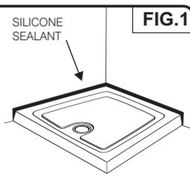
Once the walls have been tiled but **before** the enclosure is installed, the tiles **must** be silicone sealed to the tray all of the way around in one continuous bead.
