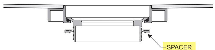
**6** Screw **Rubber Sealing Bung** to the **Threaded Connector** and fully hand tighten, ensuring that the rubber seal is towards the underside of the shower base.
