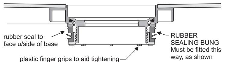
**7** Fit base into Metal Tray as described in the Aqua4MA Installation Instructions. Connect **Inner Cup** to **Inner Tube** and insert into the waste.
