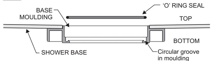
**4** Insert **Threaded Connector** into the relevant waste hole.
